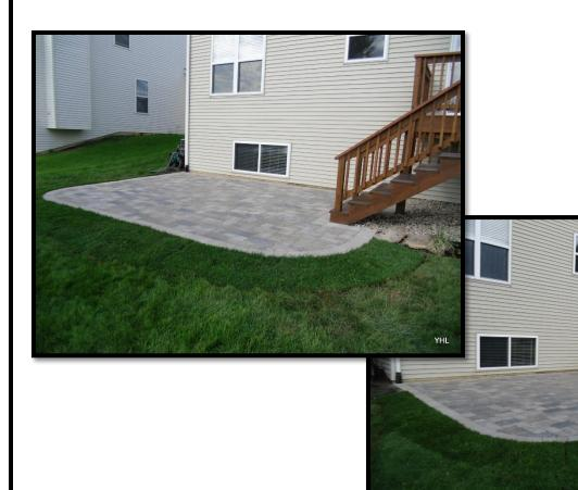
Project Scope: Unilock Brussels Block Y Pattern – Sierra with Brussels Block Half Soldier - Sandstone, yard was graded to meet patio surface, rock under deck and one downspout buried to direct water away from patio Price range does not include deck.
